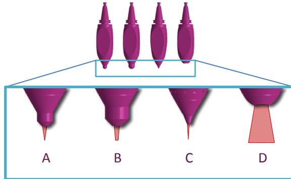
**Figure 8: Four different laser-based processing heads are shown each with a different laser profile optimized for A) fine cladding B) high rate cladding C) laser hole drilling and D) divergent focus for area pre-heating, annealing, or heat treatment**
