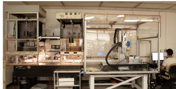
**Figure 3: Multi-material, multi-technology FDM which shuttles the part platform back and forth to achieve the combined use of multiple technologies (and multiple materials) in a single build (Image courtesy of Ryan Wicker, University of Texas at El Paso and described in [25])**
